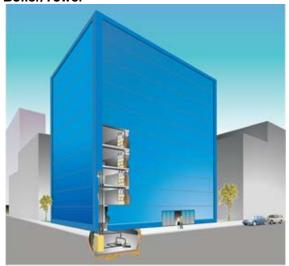
Also called a standard, conventional or water loop system, a boiler/tower system uses a two pipe water circulating system to add, remove, or transfer rejected heat to other units throughout the building. The system is not geothermal – it typically uses a natural gas or electric boiler located in a mechanical equipment room to provide heat. A cooling tower is used to dissipate waste heat. This system is typically the lowest cost of the loop options. (ARI 320 / ISO 13256-1)
