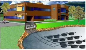
Surface water closed loop geothermal systems use a loop that is directly installed in a lake or pond near the building, making it an extremely efficient and cost effective. Bundled polyethylene coils are used in a reverse return design. Care must be taken to ensure the body of water will meet building loads. Debris problems from flooding or the need for public access may limit the use of this application. (ARI 330 / ISO 13256-1)
