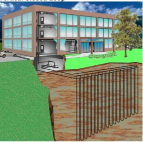
Vertical loop geothermal systems are ideal for projects with minimum available space. Vertical bore holes are drilled150 to 400 feet deep depending on building design considerations. A plastic polyethylene supply/return pipe is inserted into the holes and wells are connected in a parallel reverse return arrangement to allow water to circulate evenly throughout the bore field. Loop temperatures range from 37°F to 95°F. (ARI 330 / ISO 13256-1)
