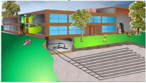
Horizontal loop geothermal systems use a series of parallel loops are installed in trenches approximately 5 feet below the ground. The piping may be installed using a "four-pipe" or "six-pipe" design. This system is well suited for applications where physical space is available – between 1,500 and 2,000 square feet/ton of cooling is required – or where bore drilling is prohibitive. (ARI 330 / ISO 13256-1)
